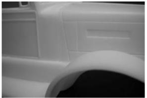
If you install an air cleaner, ensure that you scribe a new vertical body line on the side that the air cleaner will be mounted. This will separate the air cleaner hose insert panel from the hood side panel, as shown above.
