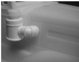
Cement the air cleaner top (large or small cap) to air cleaner housing, but don't attach the elbow yet. Cement the air cleaner to the right side of the cab, being sure to use the elbow as a guide to ensure proper alignment.
