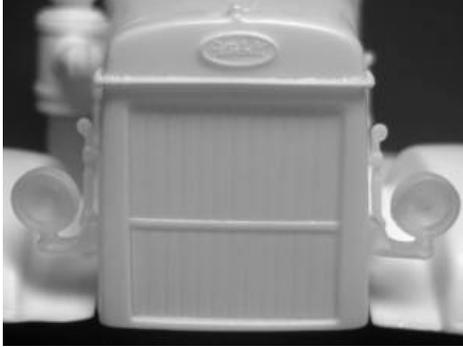
You might have to file/sand the edges of the headlight lenses to ensure a proper fit inside the headlight housings.
