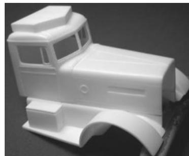
Make sure that the bottom of the cab is flush with the inside of the fenders, so that the interior tub will fit inside the cab later.
