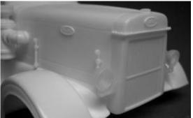
2 hood latches are needed for each side of the hood. Cement with the round portion at the top. Emblems are placed at the top of the butterfly hood side, roughly 2 scale inches (1/25-scale, or centered) from the radiator.
